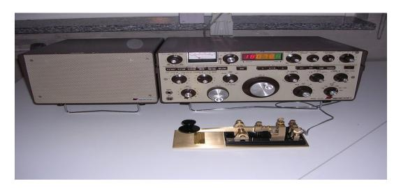
The Galaxy R-350 receiver featured a novel phase-locked loop (PLL) that provided exceptional freque ncy stability. The Inoue FDFM 2 Meter, 6 channel FM transceiver signaled the introduction of the Japanese manufacturers into the VHF region.
